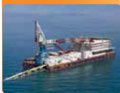
Shallow water pipe lay
