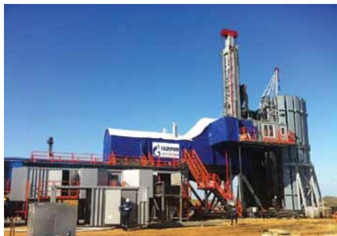
The most evident characteristic of the HH Rigs is the self-erecting hydraulic telescopic mast, made of one powerful hydraulic cylinder. The mast has an integrated hydraulic top drive built in. It is a self-standing telescopic mast with reduced height, suitable to handle range 3 "supersingles" drill pipes.
